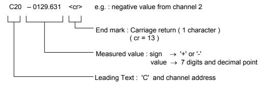
It is also possible to receive a '**TO**' message instead of a measured value. This message appears, if no gauge is connected or the gauge is not ready to operate.
